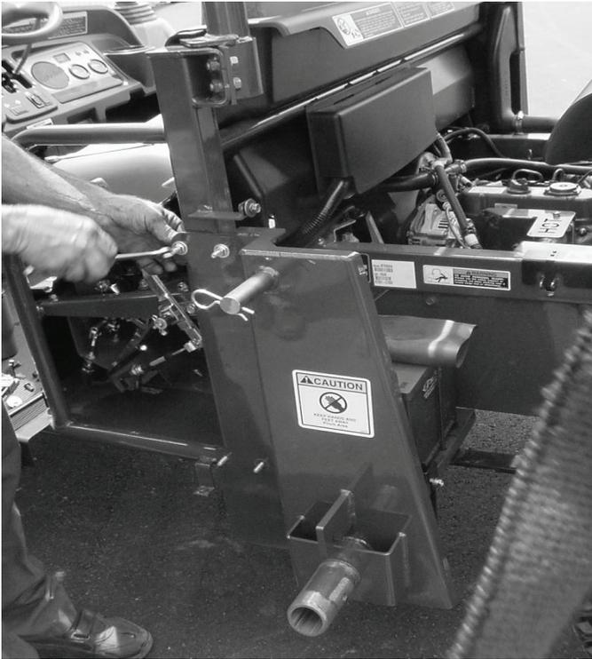
Step 2. Locate the upright 2" square tubing and install two 2"x3/8" U-bolts. Only snug do not tighten.
