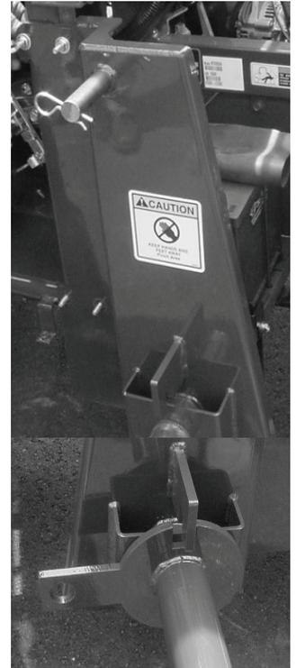
Step 5. Install cylinder and hoses. Be sure to route the hoses through the hand holder at back of bed. (NOTICE: Unit must have hydraulics for edger to work properly)
