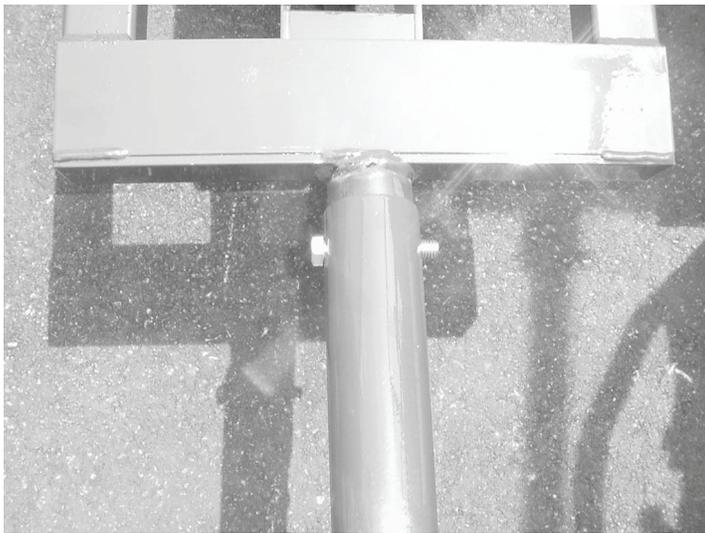
Step 6. Install main coulters frame into control arm using a 1/2"x3" bolt and nut. Reinstall left cover.
