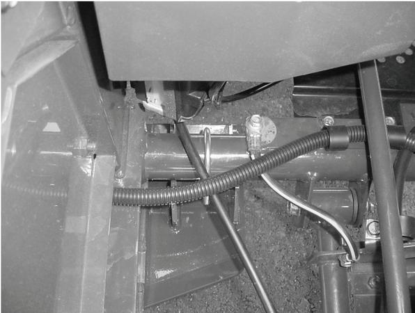
Step 3. Install a 2"x3/8" U-bolt to bottom of spring shackle tube. Tighten and then tighten the other U-bolts.
