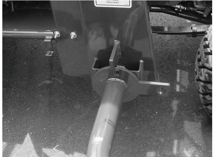
Step 4. Install control arm by lining up capture point. Control Arm will point towards the front when locked in.
